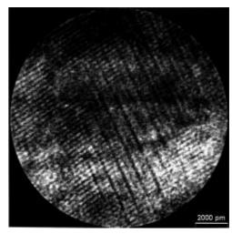
**Fig. 8.** The high-resolution TEM picture taken on the La<sub>0.8</sub>Sr<sub>0.2</sub>Fe<sub>0.3</sub>Co<sub>0.7</sub>O<sub>3</sub> sample shows an anisotropic ordered perovskite-type structure.
