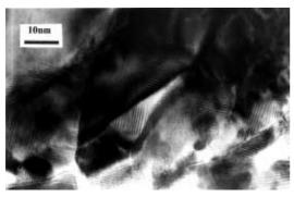
Fig. 5. TEM picture of the characteristic domain structure detected in the La<sub>0.8</sub>Sr<sub>0.2</sub>Fe<sub>0.05</sub>Co<sub>0.95</sub>O<sub>3</sub> sample.
