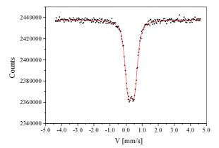
**Fig. 9.**  $^{57}$ Fe Mössbauer spectrum of La<sub>0.8</sub>Sr<sub>0.2</sub>Fe<sub>0.3</sub>Co<sub>0.7</sub>O<sub>3</sub> taken at 290 K.
