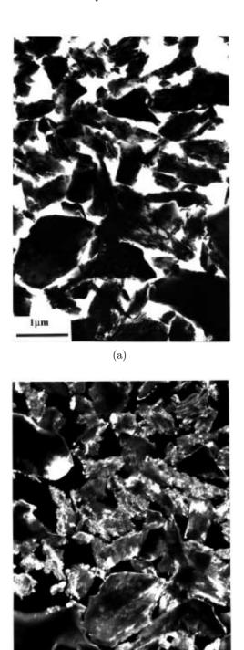
**Fig. 3.** Conventional TEM pictures taken in (a) bright-field and (b) dark-field mode on the  $\rm La_{0.8}Sr_{0.2}Fe_{0.025}Co_{0.975}O_3$  sample.
