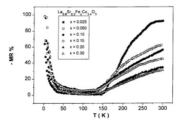
**Fig. 1.** Magnetoresistance (MR) ratio versus temperature for La<sub>0.8</sub>Sr<sub>0.2</sub>Fe<sub>x</sub>Co<sub>1-x</sub>O<sub>3</sub> (x=0.025-0.3) compounds at a magnetic field of 7.5 T [1]. The magnetoresistance was defined as MR = [R(H) - R(0)]/R(0) where R(H) and R(0) refer to the resistance in a magnetic field H and in zero magnetic field, respectively.
