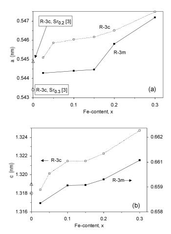
Fig. 2. Lattice parameter values derived from the XRD patterns of the  $\text{La}_{0.8}\text{Sr}_{0.2}\text{Fe}_x\text{Co}_{1-x}\text{O}_3$  samples. The open symbols refer to a fitting to a rhombohedral crystal structure with the R-3c space group and the filled symbols to a slightly deformed cubic perovskite type crystal structure with the R-3m space group. The open triangle and circle refer to the iron-free compound lattice parameters for the Sr-contents as indicated from reference [3].
