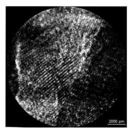
**Fig. 4.** Atomic resolution TEM picture taken on the  $La_{0.8}Sr_{0.2}Fe_{0.20}Co_{0.80}O_3$  sample.
