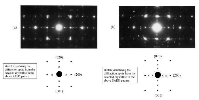
Fig. 6. Typical SAED patterns taken on the  $La_{0.8}Sr_{0.2}Fe_{0.05}Co_{0.95}O_3$  sample from the  $\langle 001 \rangle$  direction where the weak superreflection spots indicate lattice (a) doubling and (b) tripling. The sketches attached to the SAED patterns visualize which spots arise from the selected individual crystallite only.
