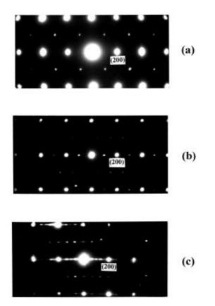
**Fig. 7.** Typical SAED patterns taken from the  $\langle 021 \rangle$  direction, where the weak superreflection spots indicate the superstructures in samples (a) at the smallest Fe-content (x=0.025) and at (b) x=0.15 and (c) x=0.30.
